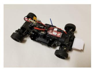
On a Mini-z 1:24 scale you can mount the transponder with sided tape.
