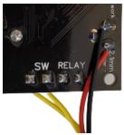
Connect Red and black wires to the back side of the Trackmate interface as shown.
