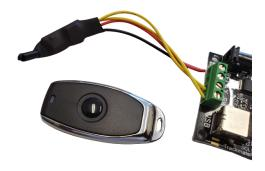
2 Yellow wires connect to the SW screws on the SCL3USB interface. You may leave the hardwired track call button wires in the screw terminals as well. Both the wired and wireless buttons can work together.
