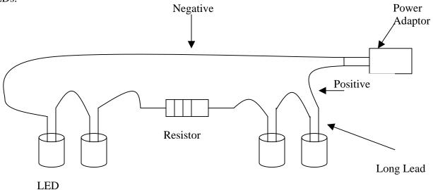
The LEDs have a short and long lead. Connect as shown. The resistor has no polarity so orientation is not important.
